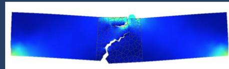
Hybrid multi-scale approach to fracture of polycrystalline materials, Akbari, Kerfriden, Bordas. *Philosophical Magazine*, 2015
