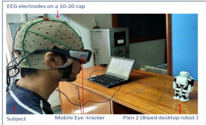
A subject interacting with a humanoid robot, during which his brain signals and Eye tracking information is aquired.
